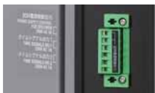
Specimen power supply control terminal, Time signals
