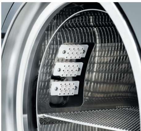
Specimen signal terminals (internal)
